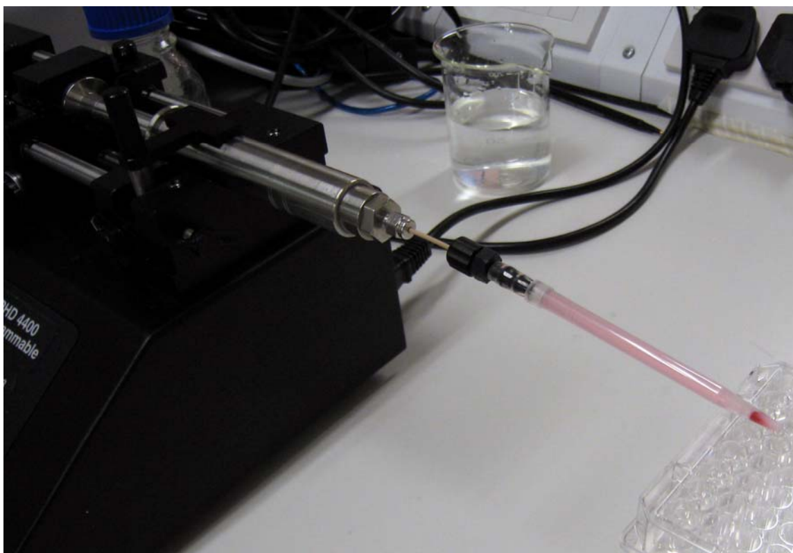
Figure 2.3 A photo shoot of the setup of the micro-scale experiment. In the image, a 50 mL syringe is set onto the pump device and the syringe is connected to a 40 \mu\text{L} pipette tip.
