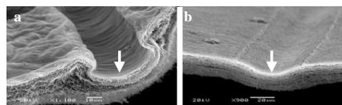
Fig. 2. SEM images of features, embossed in to the PC collagen (arrows). a- FLS, b-NFLS
