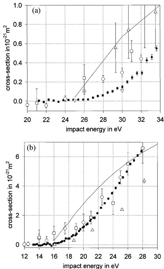
FIG. 2. (a)  $Q_i^+$  for He: filled circles, the present data; open circles [13]; open squares [26], open upward pointing triangles [14]; open downward pointing triangles [30].  $Q_i^-$  for He [28], solid line. (b)  $Q_i^+$  for  $H_2$ : filled circles, the present data; open circles [13]; open squares [26], open triangles [31].  $Q_i^-$  for  $H_2$  [27], solid line.
