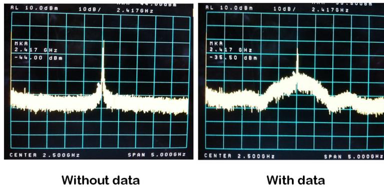
Fig. 5. Traces of the IF spectrum at 2.5 GHz.
