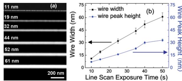
Fig. 1. (a) SEM top view image of lateral tungsten nanowires grown with a 1 pA ion beam current, using exposure time of 10, 15, 25, 35, 40 and 50s respectively; (b) wire width and peak height (measured by atomic force microscope) as a function of the exposure time.
