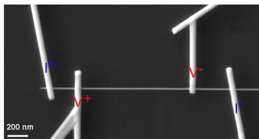
Fig. 2 SEM top view image of a typical four terminal configuration of a lateral tungsten nanowires that is 19 nm wide and 10 nm thick for electrical property measurement.
