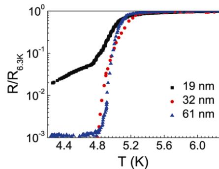
Fig. 4. Normalized resistance vs temperature of the 19, 32 and 61 nm wide nanowires with normalized resistance in the log plot, showing distinct transition characteristics.
