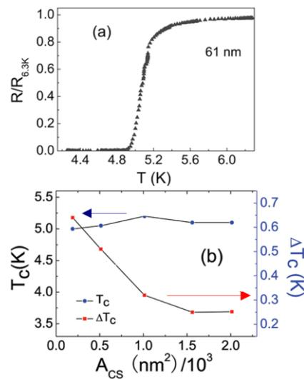
Fig. 3. (a) The temperature dependent normalized resistance of the tungsten nanowires that is 61 nm wide; (b) superconducting transition temperature ( $T_c$ ) and transition width ( $\Delta T_c$ ) as a function of the cross-sectional area ( $A_{CS}$ ) of the nanowires.
