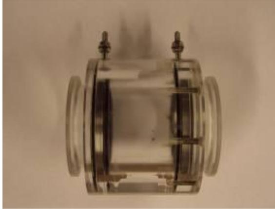
**Figure 3.9:** Conductivity ring probe for phase continuity measurement at the pipe periphery.
