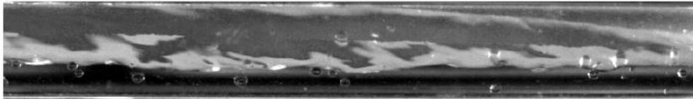
**Figure 2.3:** Dual continuous flow with several oil drops entrained in the water continuous layer. (Ngan et al., 2007)
