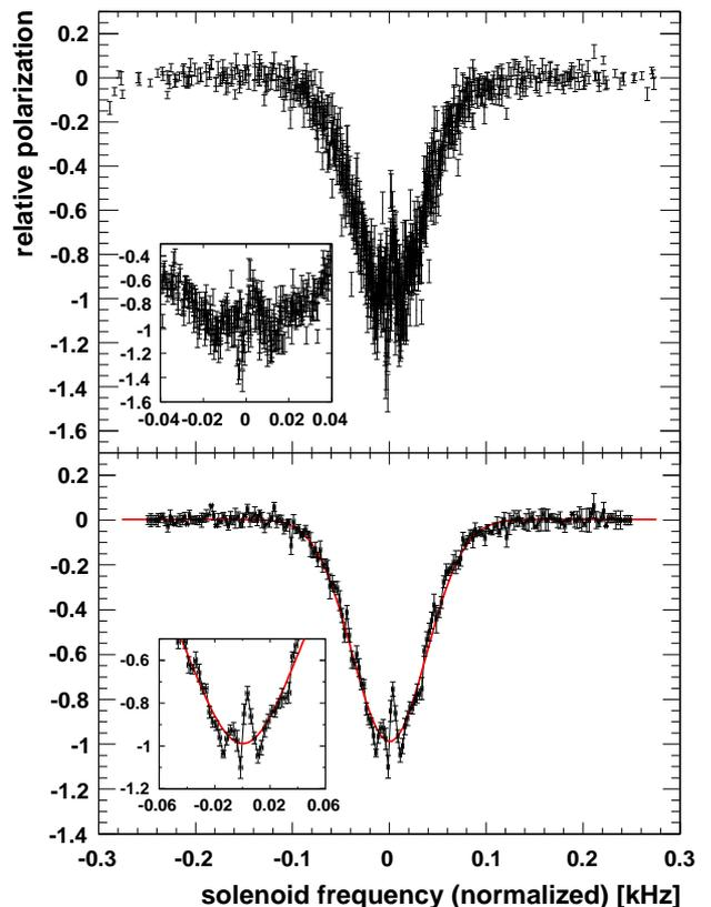
**Fig. 3.** Panel (a): The spin resonance spectra normalized by a gaussian. Panel (b): The same but with a binned abscissa in addition. The spin resonance shape is symmetric about zero and smooth except in the center, where a double peak structure is seen. This arises from the synchrotron oscillations of the beam particles caused by the interaction of the deuteron beam with the *bb* cavity. The inserts show the resonance valley in greater detail.
