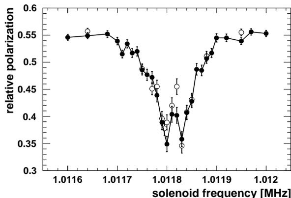
**Fig. 2.** Spin resonance measurements at one energy (closed circles). The open symbols represent results obtained for an extended cycle time, where the perturbing solenoid was switched on after 178 s.
