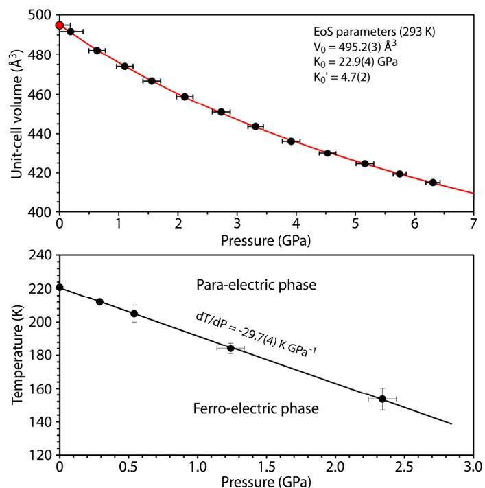
**Figure 2:** Observed pressure dependence of the para- to ferro-electric phase transition in deuterated ammonium sulfate.
