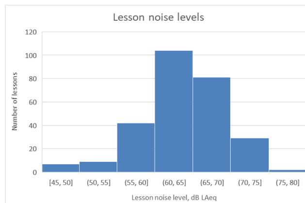
Figure 1. Histogram of equivalent continuous noise levels measured during 274 secondary school lessons
