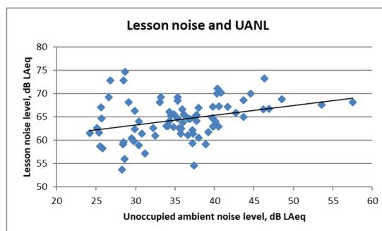
Figure 2. Relationship between occupied and unoccupied classroom noise levels<sup>1</sup>
