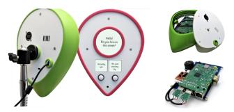
Figure 2. Design of the *Pin* devices: form, interface and hardware.
