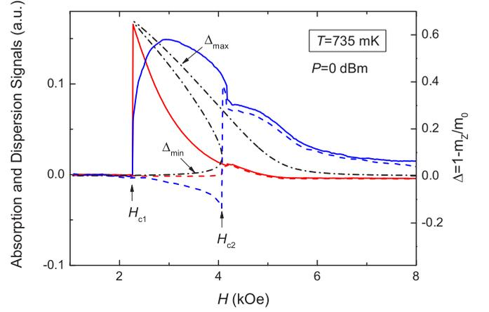
FIG. 6. Absorption and dispersion signals measured at  $T = 735$  mK at the highest input rf power of  $P = 0$  dBm during up-field (dashed lines) and down-field (solid lines) sweeps. The dashed-dotted line is the result of numerical calculations for  $\Delta = 1 - m_z/m_0$  as described in Sec. III C.
