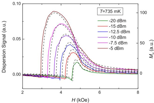
FIG. 5. Dispersion signals measured in  $\text{MnCO}_3$  at  $T = 735$  mK and at several values of input rf power (shown in the figure) during a down-field sweep. Dashed lines represent values of  $M_d$  calculated as described in Sec. III C.
