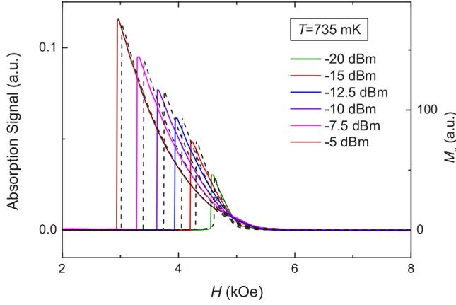
FIG. 4. Absorption signals (solid lines) measured in  $\text{MnCO}_3$  at  $T = 735$  mK and at several values of input rf power (shown in the figure) during a down-field sweep. Dashed lines represent values of  $M_a$  calculated as described in Sec. III C.
