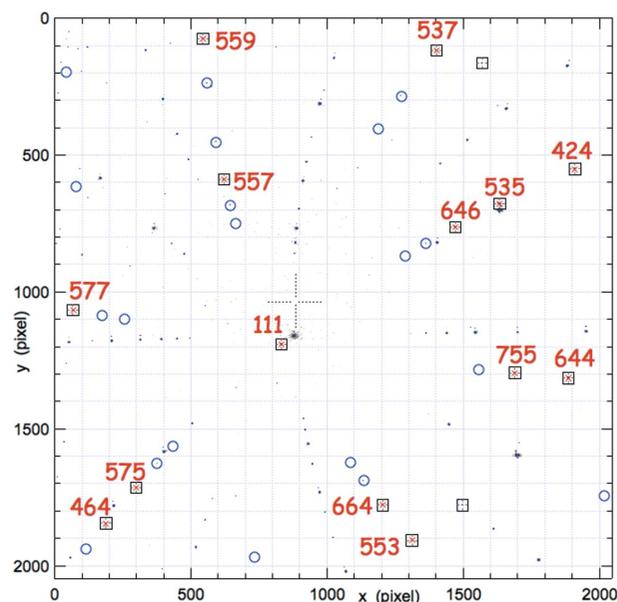
**Figure 3** Laue micro-diffraction pattern collected from the micro-crystal. Square boxes show micro-crystal reflections that were used for orientation determination. The corresponding  $hkl$  indices are shown in red. Circles represent locations where further, weaker reflections from the micro-crystal are expected. Other intense peaks in the diffraction pattern belong to the silicon substrate and are not indexed here for clarity.
