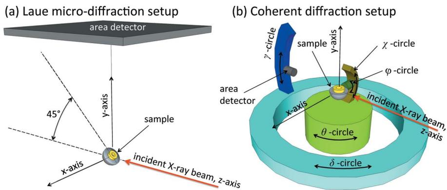
**Figure 2** Schematic of the experimental configurations for Laue diffraction (a) and coherent diffraction experiments (b). Drawings are not to scale. All coordinate systems are right-handed. Rotations in (b) are shown in their  $0^\circ$  positions.
