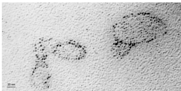
Figure 1.12 TEM image showing ring-like structures of gold nanoparticles formed on a polylysine support. Image with permission from Dai et al. 131
