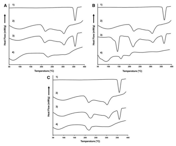
FIG. 6. (A) DSC thermograms of apigenin (1), BSA (2), physical mixture (3), and excipient-free spray-dried BSA-Api nanoparticles (4). (B) DSC spectra of apigenin (1), BSA (2), physical mixture (3), and spray-dried BSA-Api nanoparticles with lactose (4). (C) DSC spectra of apigenin (1), BSA (2), physical mixture (3), and spray-dried BSA-Api nanoparticles with L-leucine (4). DSC, differential scanning calorimetry.
