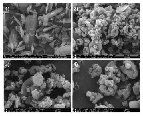
FIG. 9. Scanning electron microscopy images of raw apigenin (1), excipient-free spraydried BSA-Api nanoparticles (2), spray-dried BSA-Api nanoparticles with lactose (3), and spray-dried BSA-Api nanoparticles with L-leucine (4) 20,000 magnification.
