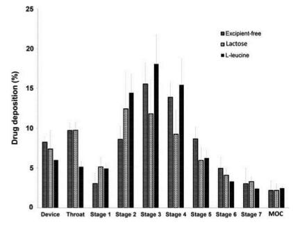
FIG. 8. Next-generation impactor deposition pattern of the spray-dried BSA-Api formulations.
