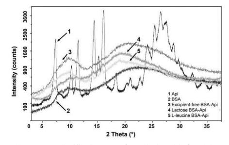
FIG. 5. X-ray powder diffraction pattern of raw apigenin and the formulations.
