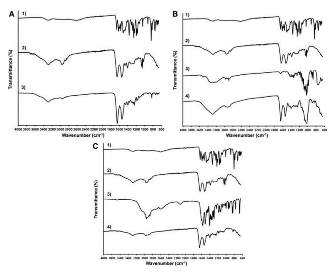
FIG. 4. (A) FT-IR spectra of apigenin (1), BSA (2), and the excipient-free spray-dried BSA-Api nanoparticles (3). (B) FT-IR spectra of apigenin (1), BSA (2), lactose (3), and spray-dried BSA-Api nanoparticles with lactose (4). (C) FT-IR spectra of apigenin (1), BSA (2), L-leucine (3), and spray-dried BSA-Api nanoparticles with L-leucine (4). FT-IR, Fourier transform infrared spectroscopy.
