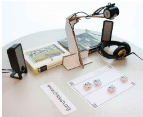
Figure 7.4: The audio d-touch basic setup – the paper surface, the labelled objects and the mounted webcam
