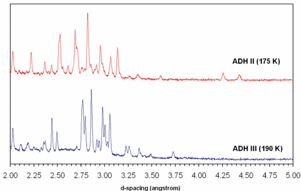
Left: diffraction patterns of ADH phases II and III collected at 5.5 kbar. The slight residual background, after subtraction of the sample environment contribution, is probably due to scattering from the silica wool.
